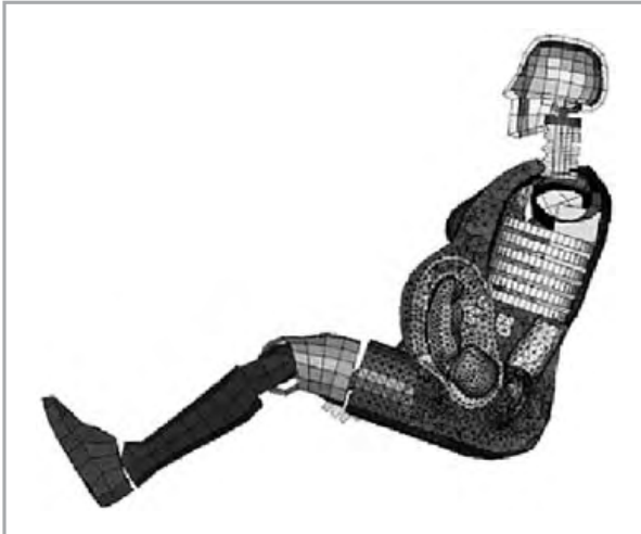
'Linda' by Volvo, the world's first virtual pregnant crash-test dummy
