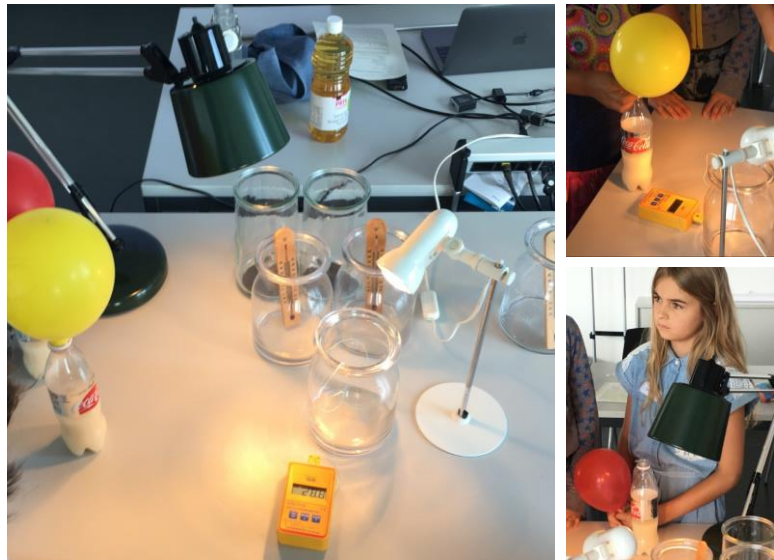
Picture 4: What is the greenhouse effect? Producing CO 2 and experiencing the change of temperature in conditions with enhanced CO 2 in a simple experimental setup
